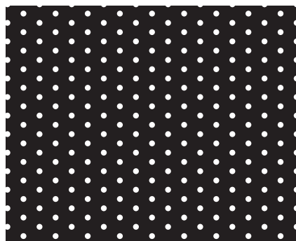
Nr. 4352 (Rv 1,1 - 3,5 / 90°) mm hole width \varnothing 1,1 pitch horizontal 3,03+3,03 pitch vertical 3,5 opening 9 % Perforation turned 90°
