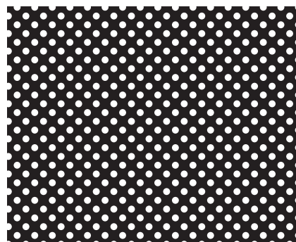
Nr. 4143 (Rd 1,3 - 2,33) mm hole width \varnothing 1,3 pitch horizontal 3,3 pitch vertical 1,65+1,65 opening 25 %
